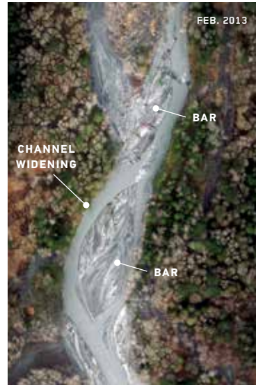
LEFT Before demolition, an artificially simplified channel; after demolition, braiding of the river as it re-engages its floodplain.
